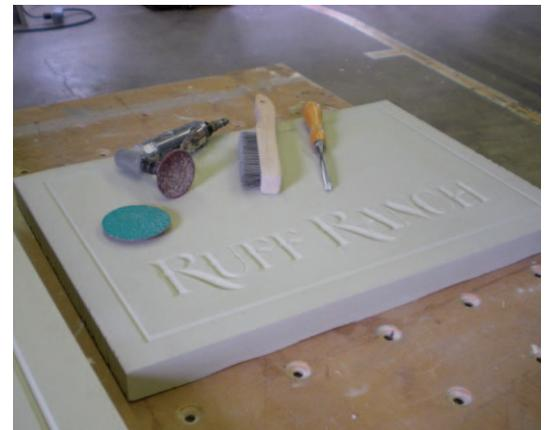
**2. CNC cut border and primary copy, both sides: 30 minutes.** Here you can see the chisel, rotary die grinder and wire brush we used for add the weathered wood grain effect.
