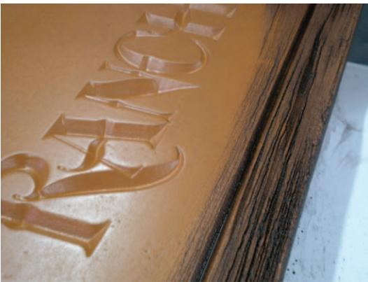
**5. Prime, paint and glaze: 90 minutes.** Applying the primer and base coat of Matthews Paint took about 45 minutes. For the glaze, we mix dark browns and black paint with 1-Shot clear, along with some 4007 hardener. We apply it to the textured portions with a rag, then wipe it back off. That keeps it darkest down in the deeper parts of the carving.
