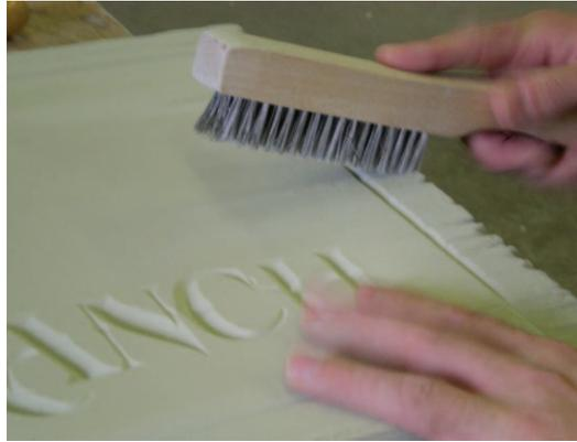
**4. Wire brushing for added depth: 60 minutes** The wire brush provides most of texture on this sign. Tapping the brush on the HDU board creates a lot of cool pores to hold the glaze.
